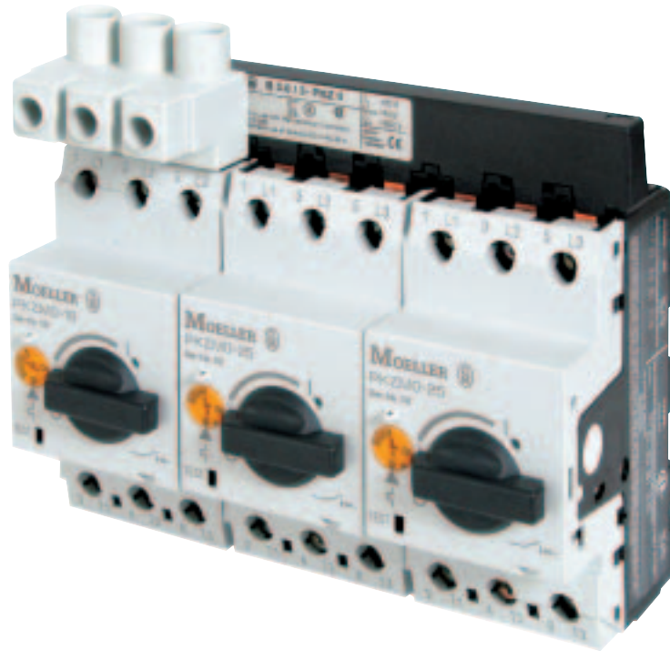
Figure 8: A group of PKZM0 manual motor controllers is linked via a commoning link bus connector. The controllers are fed by a common BK25/3-PKZ0-E terminal block. The incoming terminal's large electrical clearances at the point of supply enable the entire assembly to meet self-protected "Construction Type E" requirements.
