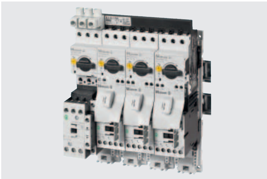
Figure 10: Example of a UL 508 Type F combination motor controller array, each consisting of a manual Type E self-protected controller and associated magnetic contactor.
