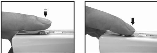
This camera is designed for 2-step shutter function. A "[ ]" mark will appear in the center of the LCD monitor when the **Shutter** button is pressed and held half way down. The camera will beep after the **Shutter** button is pressed down fully; then release the **Shutter** button to take a picture.
