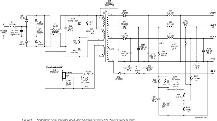
Good cross-regulation on 5 V and 3.3 V outputs is achieved by minimizing secondary leakage through the use of foil windings and by sum regulating (obtaining feedback from both outputs).
