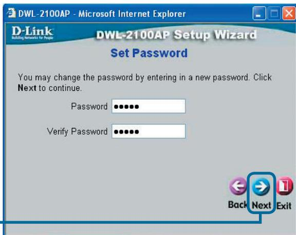
**步骤2—Wireless Setup (无线设置)**
