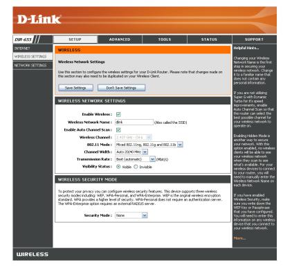
Visibility Status: Select Invisible if you do not want the SSID of your wireless network to be broadcasted by the DIR-655. If Invisible is selected, the SSID of the DIR-655 will not be seen by Site Survey utilities so your wireless clients will have to know the SSID of your DIR-655 in order to connect to it.
