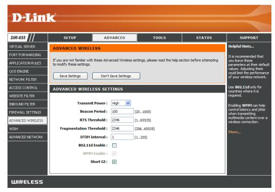
**802.11d:** This enables 802.11d opration. 802.11d is a wireless specification developed to allow implementation of wireless networks in countries that cannot use the 802.11 standard. This feature should only be enabled if you are in a country that requires it.
