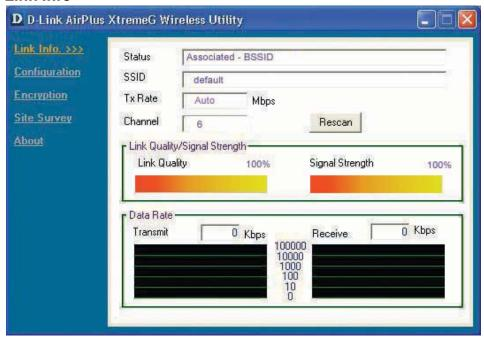
**Status:** Displays the MAC Address of the Access Point that is associated with the DWL-G650.
