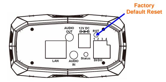
**NOTE:** Restoring the factory default setting will lose the all previous settings included IP address forever. User needs to run the IP Wizard program to search the device and configure it to let the device work properly again.
