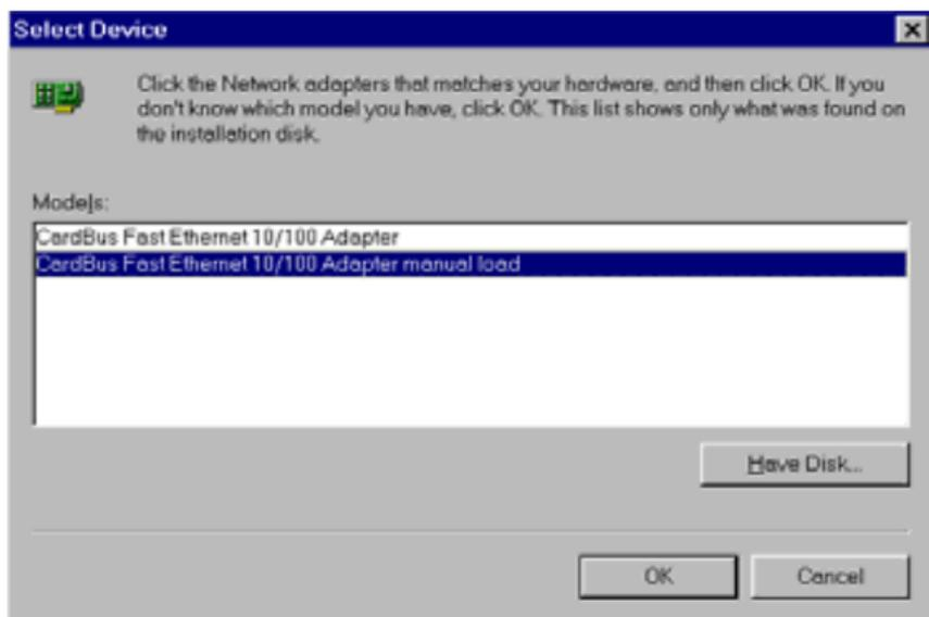
12. Click **OK**. A dialog box will appear to adjust the driver's settings. The resources assignment to adapter should be unique in the system.
