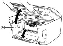
(A) Press the Open Button to open the Paper Output Tray if it does not open automatically.
