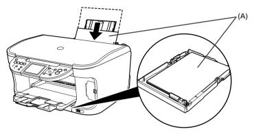
(A) If the Auto Sheet Feeder runs out of paper, the paper source automatically changes to the Cassette.
