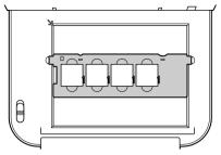
(2) Mount the slides in the film guide with the front side (the side showing the correct image) face down, the frame order running from left to right, and with the image upside down. Load the slides in the landscape orientation, making sure they are not loose in the film guide.
