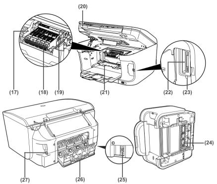
(17) Print Head Lock Lever Used to fix the Print Head.
