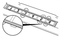
(4) With the front side of the film (the side showing the correct image) face down, align the film guide with the indentations on the right and left sides of the Platen Glass.
