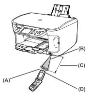
(2) Select the photo to print and send the data to the machine using the infrared communication function of the mobile phone. Printing will start after receiving all data.
