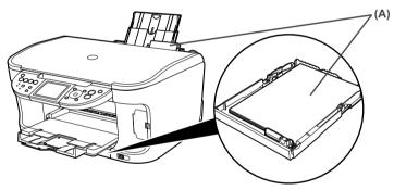
(A) You can switch between paper loaded in the Auto Sheet Feeder (e.g., 4" x 6" / 101.6 x 152.4 mm) or the Cassette (e.g., A4/Letter-sized paper).
