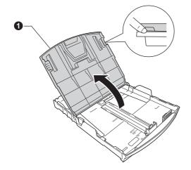
C With both hands, gently press and slide the paper side guides ● and then the paper length guide ② to fit the paper size.
