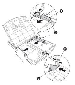
Fan the stack of paper well to avoid paper jams and misfeeds.
