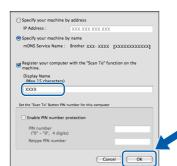
The name you enter will appear on the machine's LCD when you press the **SCAN** key and choose a scan option. (For more information, see Network Scanning (For models with built-in network support) in the Software User's Guide on the documentation CD-ROM.)
