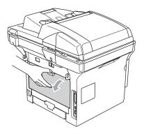
4 Pull the tabs at the left and right hand sides toward you to open the fuser cover (1).
