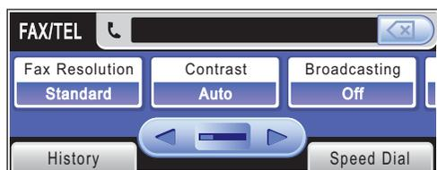
Press ◀ or ▶ to scroll through the **Fax** key options. Some functions are only available when sending monochrome faxes.
