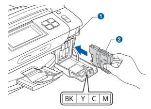
Install each ink cartridge in the direction of the arrow on the label.
