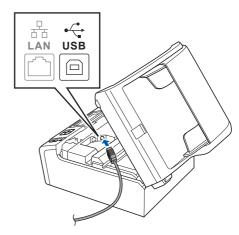
Carefully guide the USB cable through the trench as shown below, following the trench around and toward the back of the machine. Then connect the cable to your Macintosh®.
