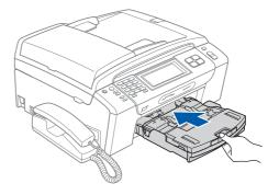
While holding the paper tray in place, pull out the paper support 1 until it clicks, and then unfold the paper support flap 2.
