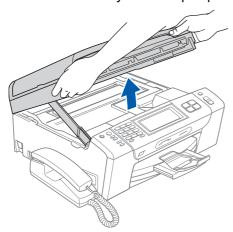
Connect the network cable to the LAN socket marked with a symbol. You will find the LAN socket inside the machine on the left as shown below.
