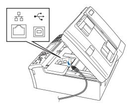
12 Carefully guide the USB cable into the trench as shown below, following the trench around and toward the back of the machine. Then, connect the cable to your computer.
