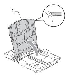
Press and slide the paper side guides (1) and paper length guide (2) to fit the paper size.
