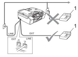
When the TAD answers a call, the LCD shows Telephone (MFC-440CN only) or Ext. Tel in Use (MFC-665CW only).
