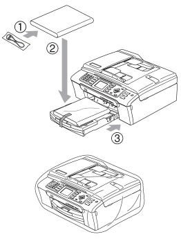
D Pack the printed materials in the original carton as shown below. Do not pack the used ink cartridges in the carton.
