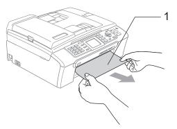
■ If you cannot remove the jammed paper from the front of the machine, or the error message still appears on the LCD after you have removed the jammed paper, please go to the next step.
