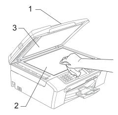
2 In the ADF unit, clean the white bar (1) and the glass strip (2) under it with isopropyl alcohol on a lint-free cloth.
