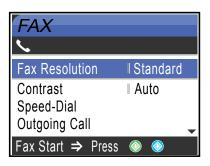
Press  $\blacktriangle$  or  $\blacktriangledown$  to scroll through the **Fax** key options. Some functions are only available when sending monochrome faxes.
