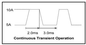
Note that this transient behavior works with any of the operation modes CC, CV, CW, or CR. Here are the keystrokes used to setup this continuous transient condition:
