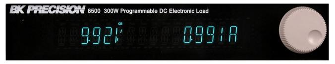
The instrument's voltage display may read a bit less than the power supply's output -- this may be due to a voltage drop in the wires connecting the power supply to the DC Load. Press the  $\triangle$  or  $\nabla$  keys to see the power that is being consumed by the load.
