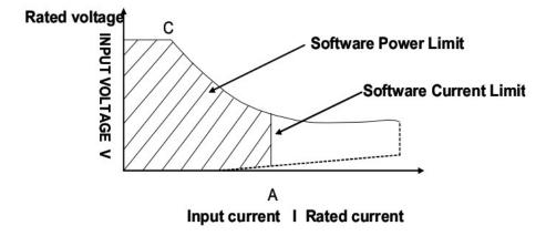
Note the gap between the operating region and the current axis for lower voltages. More detail is described in the following section.
