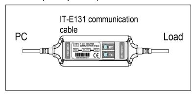
The LEDs in the adapter will blink when information is sent through the adapter. This is a good way to tell if your communication link is active.
