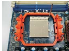
STEP 1: Lift Up The Socket Lever
