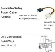
Please connect the black end of SATA power cable to the power connector on each drive. Then connect the white end of SATA power cable to the power connector of the power supply.
