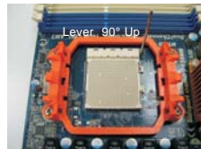
STEP 1: Lift Up The Socket Lever
