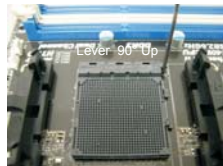
STEP 1: Lift Up The Socket Lever
