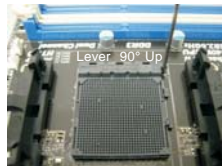
STEP 1: Lift Up The Socket Lever
