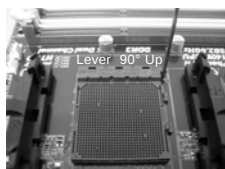
STEP 1: Lift Up The Socket Lever
