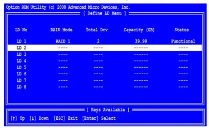
2. Press the up and down arrow keys to select an available logical drive number and press <Enter>.
