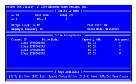
Choose the RAID level you want. In the Define LD Menu section, press the spacebar to cycle through logical drive types, including RAID 0, RAID 1, RAID 5, RAID Ready, JBOD and RAID 10.
