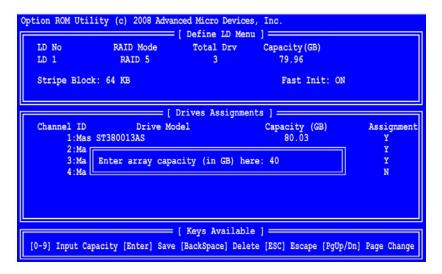
1. Enter the desired capacity (MB) for the first logical drive and press <Enter>. The Define LD Menu displays again.
