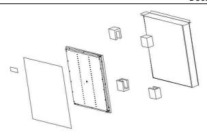
Step 2: fold the eight cartons → attach one honeycomb cardboard at each side → install lid and tray at both bottom and top side → use packing machine to fasten it up Shown as below:
