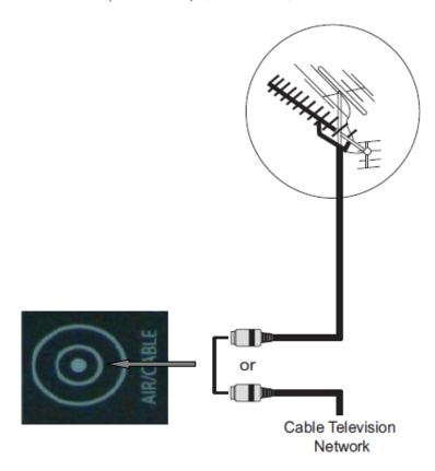
Figure 3-7. Air/Cable Connection.
