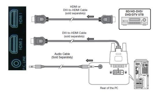
Figure 3-1. HDMI Connections
