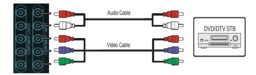
Figure 3-3. Component Video Connections
