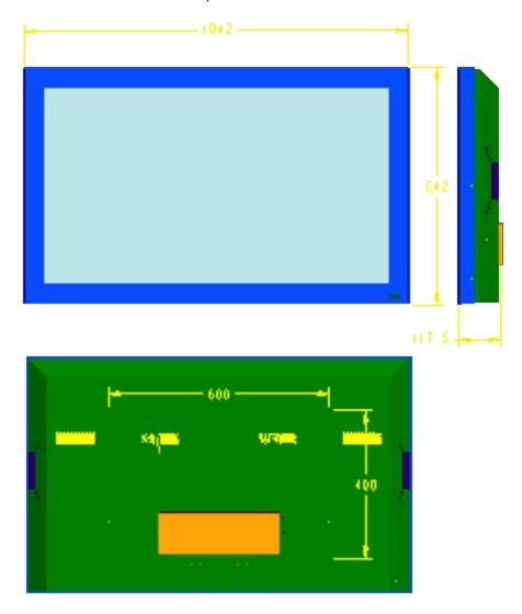
Figure 6-1. CP-42HD Dimensions (Front/Side/Rear)
