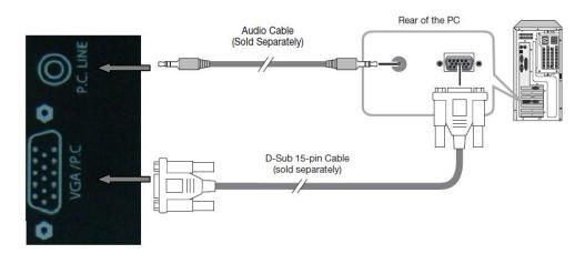
Figure 3-2. Analog RGB Connections
