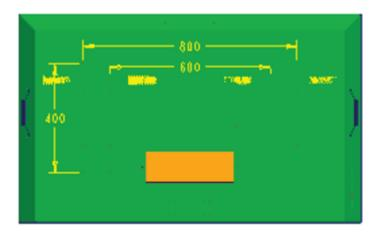
Figure 6-2. CP-52HD Dimensions (Front/Side/Rear)
