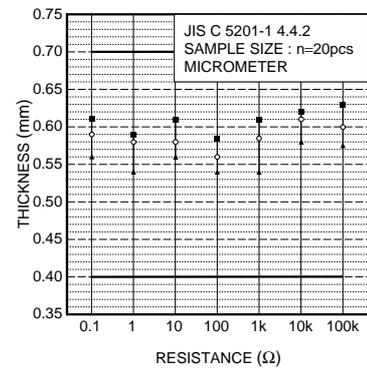
Fig.4 Dimensions (thickness)
