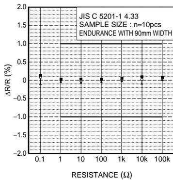
Fig.14 Bend strength of the end face plating
