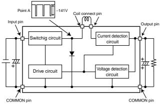
Impressing the 100V(DC conversion= 141V) rectified between Input pin-COMMON pin, Switching 0 to 141V as shown wave shape at the internal circuit point A and smoothing by output capacitor enables to output.
