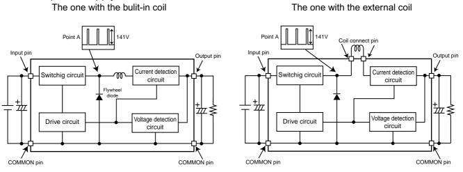
Impressing the 100V(DC conversion=141V) rectified between Input pin-COMMON pin, Switching 0 to 141V as shown wave shape at the internal circuit point A and smoothing by output capacitor enables to output.
