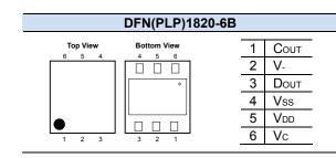
\*) The tab is substrate level (VDD)
