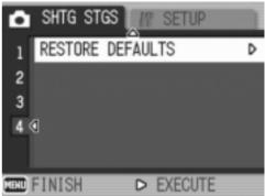
• The display indicates the camera is restoring the initial settings. Once it is finished, the display returns to the shooting mode screen.
