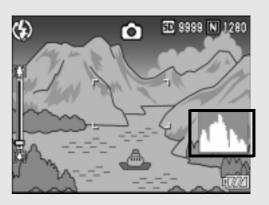
By using the histogram, you can determine the brightness of an image without being affected by the brightness around the LCD monitor. This also helps you correct for areas that are overly bright or dark.
