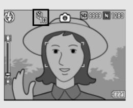
• Each press of the 𝔅 (Self-timer) button changes the self-timer setting in the following order: 10 sec, 2 sec, and Self-timer Off.
