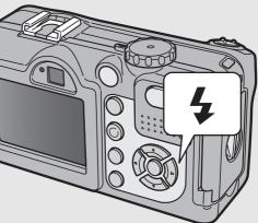
The auto focus/flash lamp blinks while the flash charges. Once the flash is charged, the lamp turns off and the camera is ready to shoot.
