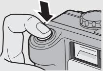
The still image you have taken appears momentarily on the LCD monitor and is recorded to the internal memory or SD memory card.
