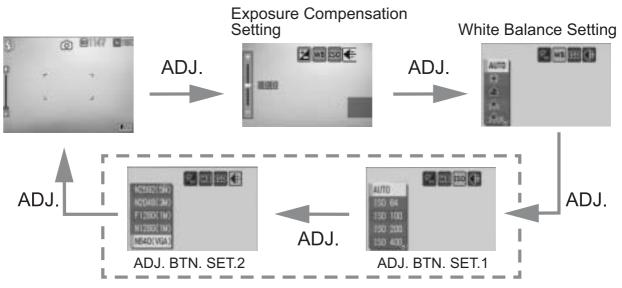
Use the SETUP menu to assign a function to ADJ BTN. SET.1 and ADJ BTN. SET.2. (PP.120)
