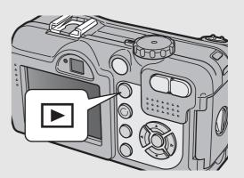
To switch the camera from Playback Mode to Shooting Mode (or Voice Memo Mode), press the ▶ (Playback) button again.
