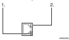
① Indicator (green)Remains green when the machine is properly connected to the network.
