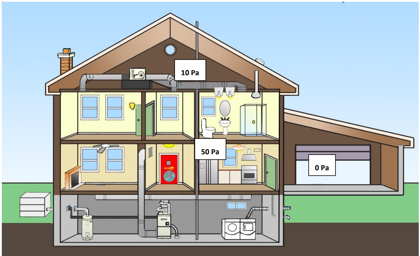
Figure 10: Zonal pressures in a home's unconditioned spaces.
