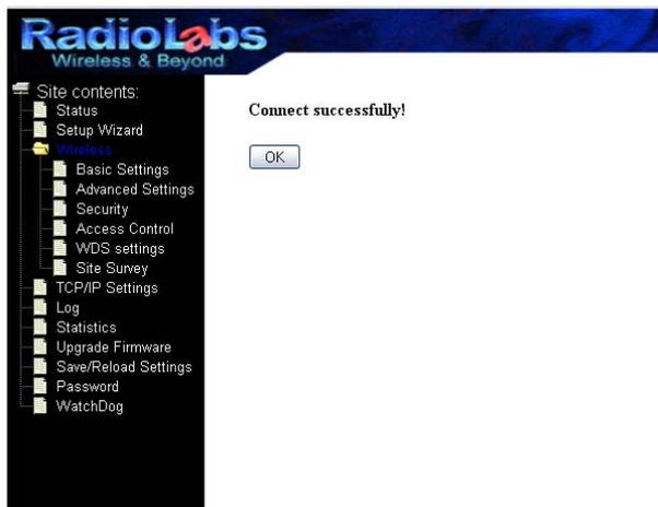
*If the encryption key or type is incorrect, the next screen will read “Encryption Type Mismatch”. You will need to recheck your security settings and try again. If the signal you are repeating is unencrypted, you need to make sure that your encryption type is set to “None” before connecting.*
