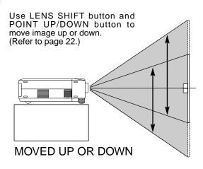
Picture tilt and projection angle can be adjusted by rotating ADJUSTABLE FEET. Projection angle can be adjusted up to 6.9 degrees by rotating Adjustable Feet.
