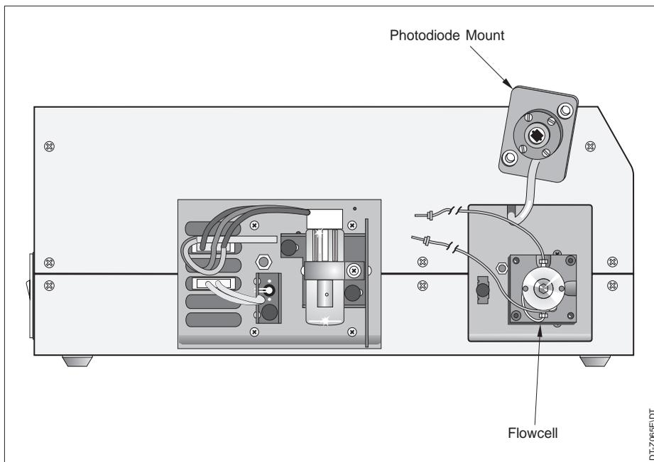
*Figure 5 ProStar 345, Inside the Side Enclosure*
