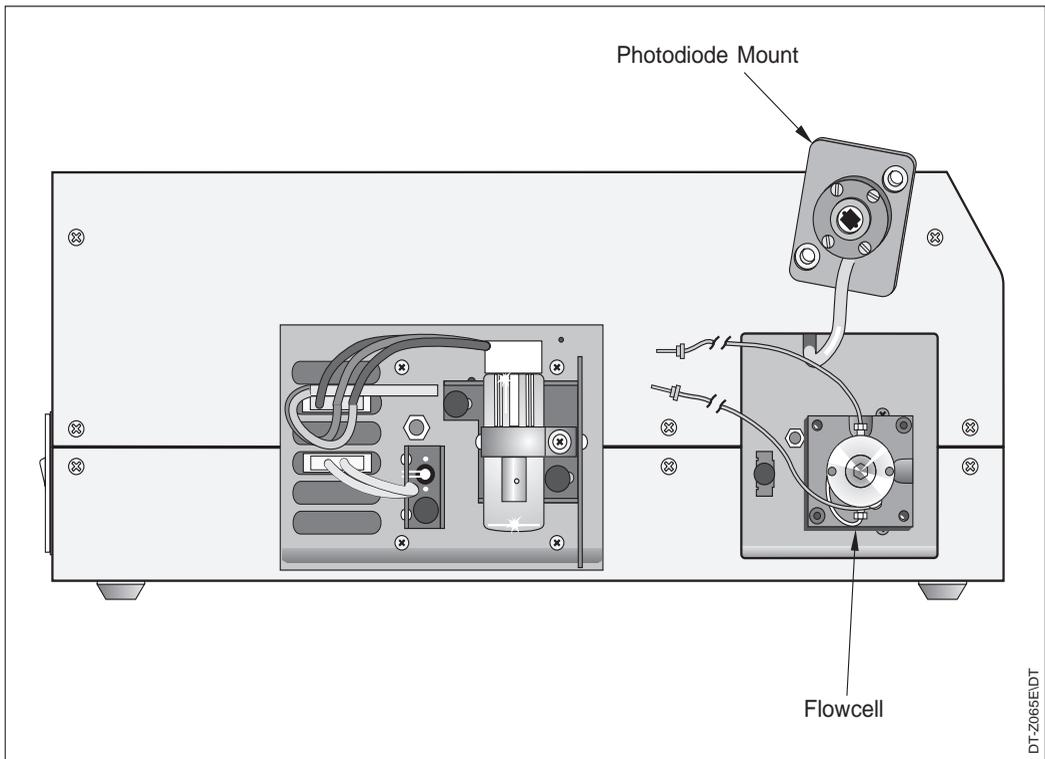
Figure 15 Repositioning the Photodiode Mount to Expose the Flowcell
