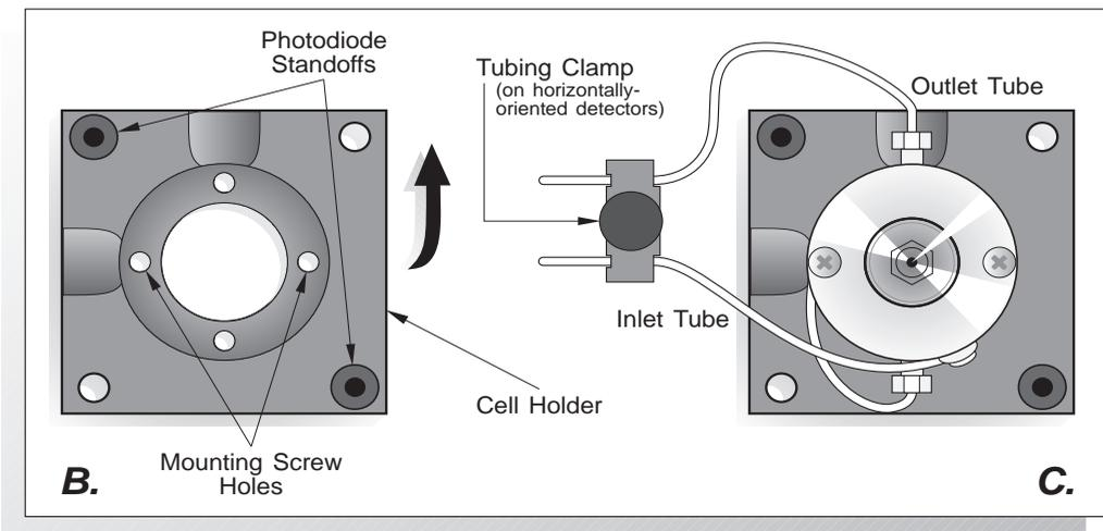
*Figure 7 Changing the Alignment of a Vertically-Oriented Flowcell*
