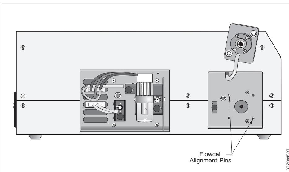
*Figure 16 Location of the Flowcell Alignment Pins*
