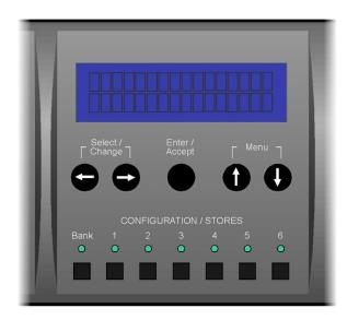
The Menu Panel provides manual control and inspection of all the ADA-8XR's operating parameters, and also contains the Configuration/Stores buttons for loading and saving setups of the ADA-8XR.
