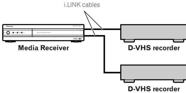
Using i.LINK cables you can also connect up to two D-VHS recorders in a daisy chain.
