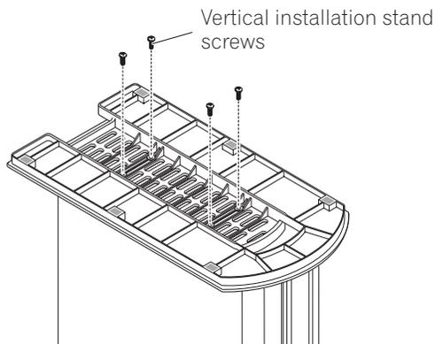
Plug the screw holes using the caps provided.
