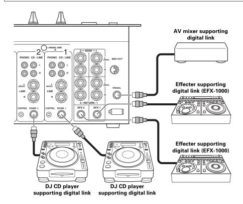
By connecting a single dedicated cable (digital link cable), exchange of audio signals and control signals can be performed digitally (The connection of audio cables or control cables is unneeded).
