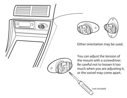
If you need to remove the mount, carefully lift the adhesive pad with your fingers or a spoon. Warming with a hair dryer for several minutes will help soften the adhesive.
