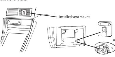
2. Attach the car cradle to either mount by sliding it into place.
