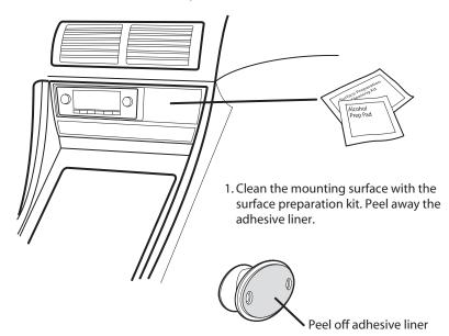
2. Firmly press the swivel mount to the surface for 30 seconds. Allow 24 hours before using the mount.
