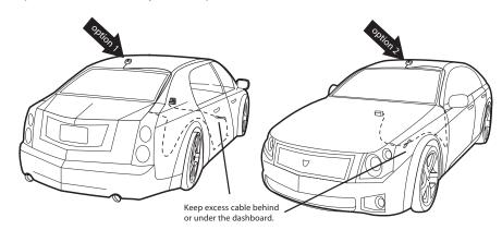
Mount the antenna to the roof or trunk of the vehicle. During installation, make sure you are outdoors and not obstructed by tall buildings.
