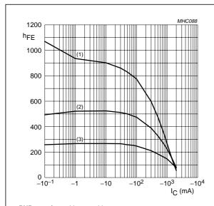
**PNP transistor;**  $V_{CE} = -5 V$ .
