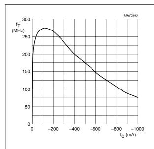
PNP transistor;  $V_{CE} = -10 \text{ V}.$
