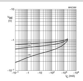
**PNP** transistor;  $V_{CE} = -5 \text{ V}$ .
