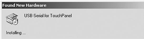
First, PC is started, and then Windows is started. The CD-ROM with USB driver software is inserted into the CD-ROM drive. Next, touch panel and PC are connected with a USB cable. (see page 10)
