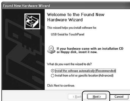
First, PC is started, and then Windows is started. The CD-ROM with USB driver software is inserted into the CD-ROM drive. Next, touch panel and PC are connected with a USB cable. (see page 10) When a USB cable is connected, the wizard of the driver setup starts.
