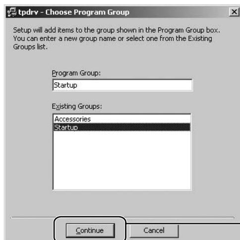
In the default, it is registered as the startup program. The driver software will start up automatically the next time the unit is turned on.
