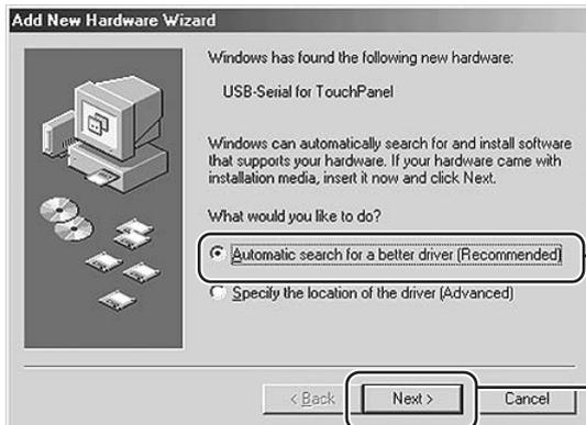
First, PC is started, and then Windows is started. The CD-ROM with USB driver software is inserted into the CD-ROM drive. Next, touch panel and PC are connected with a USB cable. (see page 10) When a USB cable is connected, it is recognized as a new hardware, and a message is indicated.
