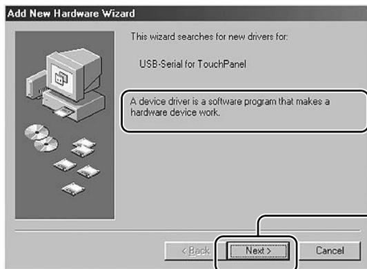
First, PC is started, and then Windows is started. The CD-ROM with USB driver software is inserted into the CD-ROM drive. Next, touch panel and PC are connected with a USB cable. (see page 10) When a USB cable is connected, "Add New Hardware Wizard" is indicated.
