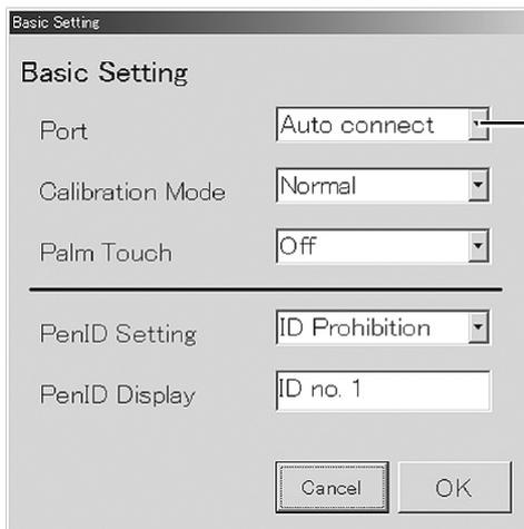
When “Auto connect” is chosen, driver software detects it automatically, and it is set up.
