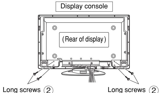
Securely fasten using long screws ②.
