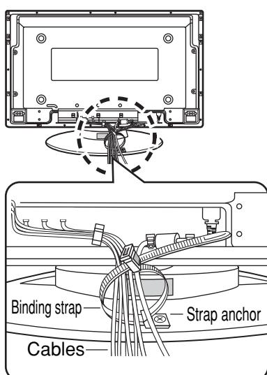
While ensuring there is sufficient slack in the cord to minimize stress, firmly bind all cables with the supplied binding strap.
