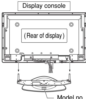
Position the side of the pedestal with the model no. label to the rear. Push the assembly into the display until it stops.
