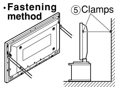
\* Securely attach to a wall, pillar or similarly solid structural feature using separately-obtained products such as cords or chains of adequate strength.
