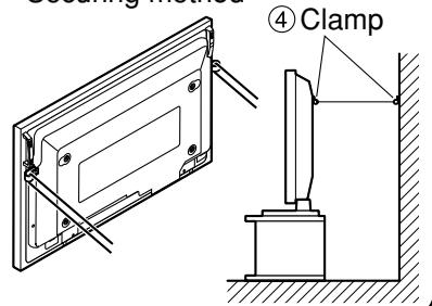
\* Use strong wire or chain which is commercially available to secure the Wide Plasma Display to a solid area of the wall or a pillar.
