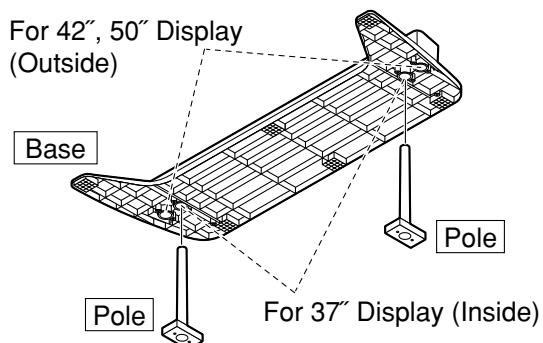
Insert the poles into the left and right holes in the underside of the base so that they fit securely as shown in the illustration above.
