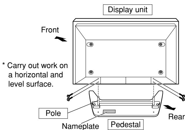
Use the assembly screws ② (Black screw) to fasten securely.
