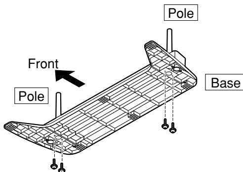
Use the assembly screws ① to secure the poles firmly to the bottom of the base.
