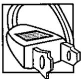
◦ A polarized power plug (two blades, one wider than the other) will fit into a power receptacle only one way. This is a safety feature. Do not defeat it. If you are unable to insert the plug fully, try reversing it, or have an electrician change the receptacle. If you
