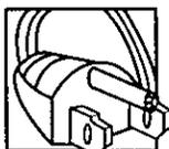
◦ A grounding type power plug (two blades and a round pin) will fit only into a grounding type receptacle with matching openings. This is a safety feature. Do not defeat it. You may need an electrician to install a grounding type receptacle. If you need an extension cord, use
