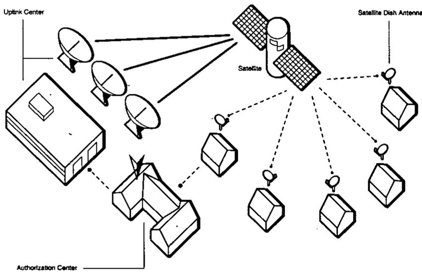
**Uplink Center** Transmits programming up to the satellite.
