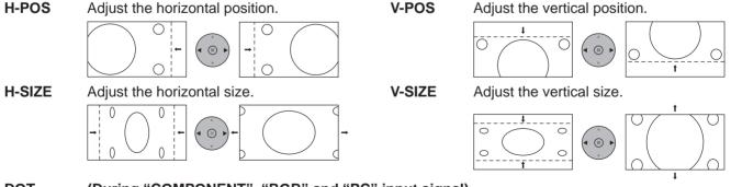
DOT (During "COMPONENT", "RGB" and "PC" input signal)
