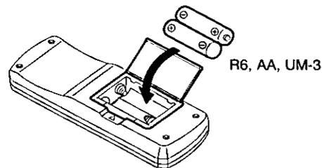
Insert the batteries observing the correct polarities (+, -).
