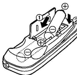
Insert the batteries observing the correct polarities (+, -)
