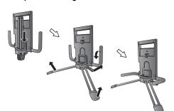
2 Install the unit on the setting stand. Align and put the unit on the setting stand, turn the screw clockwise to secure the unit
