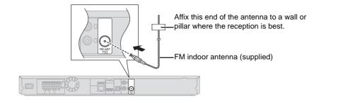
• Use an FM outdoor antenna if radio reception is poor.
