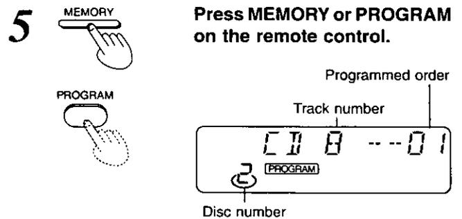
If you enter non-existing disc(s) or track(s) in the program contents, the corresponding indicator illuminates and the entry is included in the count. In the play mode, the changer will cancel the non-existing entry.
