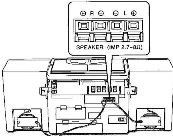
3. When using the unit with the speakers attached, wind the speaker cables as shown above.
