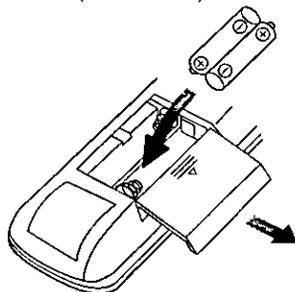
To remove the batteries, pull out the ⊕ side.
