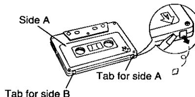
To re-record on a protected cassette, cover the slot with adhesive tape.
