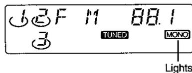
To return to stereo reception, repeat the same procedure and turn off the MONO display.
